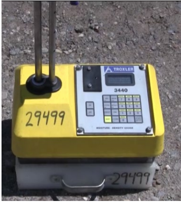
Standardizing the nuclear density gauge
